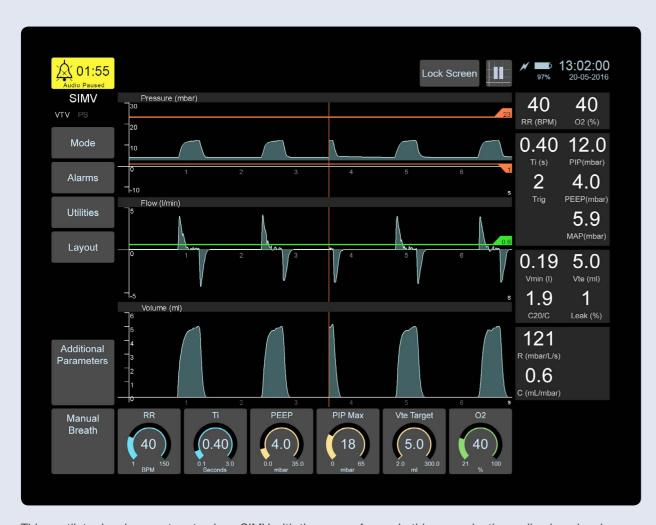
This ventilator has been set up to show SIMV with three waveforms. In this example, the audio alarm has been pre-silenced and a countdown timer within the button shows the remaining time. By default only the necessary parameters to control SIMV are visible.
